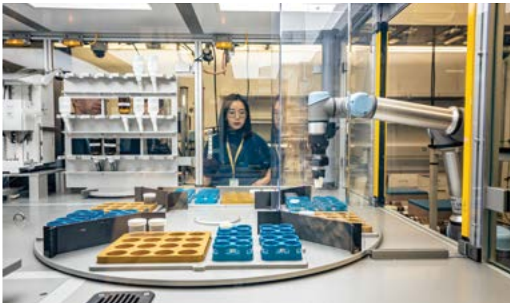
FIGURE 5.6 The A-Lab combines AI-guided synthesis with automated materials characterization
