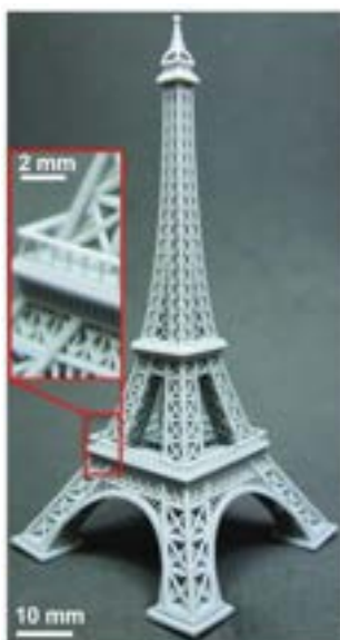
FIGURE 5.3 A CLIP-based 3-D printer created a miniature print of the Eiffel Tower
